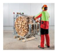
the sawing cage can be adjusted to 25, 33, 50, 66, 75 and 100 cm as standard. Loading and unloading can be performed by hand or conveniently with a front loader. The
